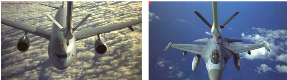
Figure 1: Flying Boom in the pre-contact position with an A330 MRTT receiver (left). Boom coupled with an F-16 receiver (right).
